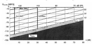
Figure 5: Dynamic range of a digital microphone
